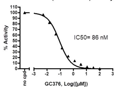
Inhibition of 3CL Protease enzyme activity by GC376, measured using the *Fluorogenic 3CL Protease Assay Kit (BPS Bioscience #78015)*. Fluorescence intensity was measured using a Tecan fluorescent microplate reader. *Data shown is lot-specific. For lot-specific information, please contact BPS Bioscience, Inc. at info@bpsbioscience.com*
