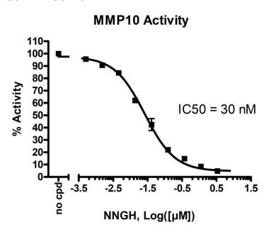
Inhibition of MMP10 enzyme activity by NNGH, measured using the *Fluorogenic MMP10* Assay Kit (BPS Bioscience #79986). Fluorescence intensity was measured using a Tecan fluorescent microplate reader. Data shown is lot-specific. For lot-specific information, please contact BPS Bioscience, Inc. at <a href="mailto:info@bpsbioscience.com">info@bpsbioscience.com</a> OUR PRODUCTS ARE FOR RESEARCH USE ONLY. NOT FOR DIAGNOSTIC OR THERAPEUTIC USE.
